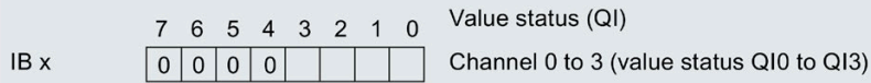
Figure 3-4 Address space for configuration as a 4-channel DQ 4x24VDC/2A HS with value status
