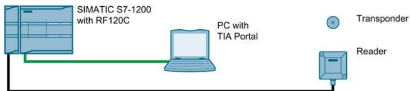
Figure 2-4 Example of integrating a SIMATIC S7-1200 with RF120C
